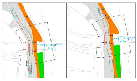
Figure 48. Riverside Drive - Shuttle Working Design Swept Paths
