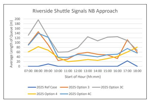
Figure 51. Average Northbound Queue Length on approach to Riverside Drive Shuttle Signals
