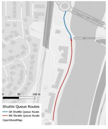
Figure 49. Queue Routes on Approach to Shuttle Signals
