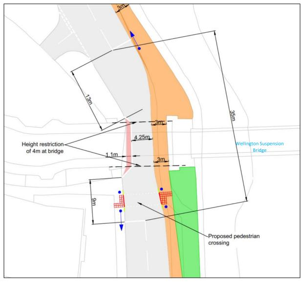
Figure 52. Riverside Drive - Shuttle Working design with Pedestrian Crossing
