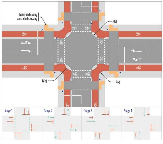
Figure 18. Example of a Protected Junction (Cycling by Design 2021)
