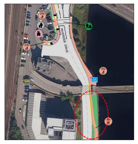
Figure 44. Phase 1 Works – Footway Re-alignment
